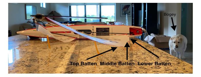
Jib Boom Adjustment - With the sheets full in, adjust the jib sheet so the end of the boom is over the first angle of the deck.
