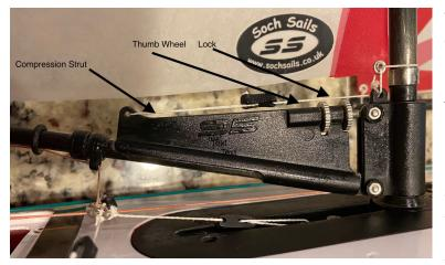
With the boom adjusted to the corner of the cockpit and your battens in the three different positions, your main is set. Twist the lock away from the mast to lock your compression strut.
