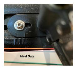
Mast Gate – this requires a small allen wrench. Your mast setting should be almost fully back 7 or 8. (Mine is all the way back - 8). For the A rig, set it and forget it.
