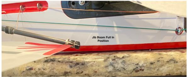
Jib Twist - Now adjust the jib topping lift so the sail twist is matching the sail twist in the main. Making the topping lift shorter will increase sail twist, longer will flatten the sail. Each adjustment will slightly change the sheet position and making large adjustments on the topping lift will change the tension on the back stay.
